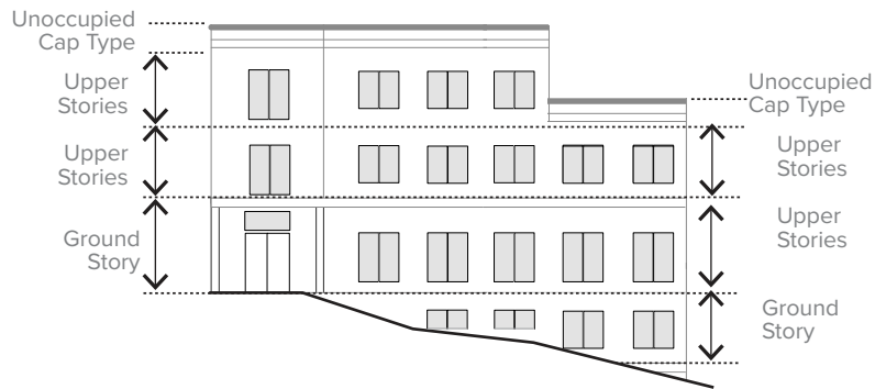
Figure 660(38) Measuring Height along Sloped Street
