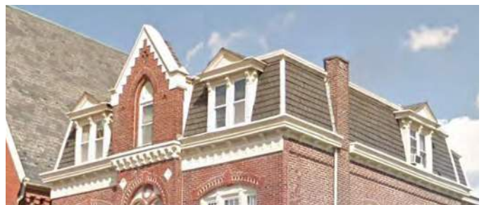
Pitched Roof Type (Mansard Roof)
