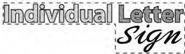
Figure 660(28) Channel Letter and Painted Wall Sign Measurement
